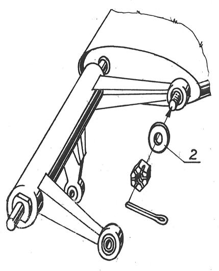
In countershaft on the stabiliser the swinging bearing is expanded. The pin of elevator is put in this bearing and is screwed in with aid of a castle nut.
